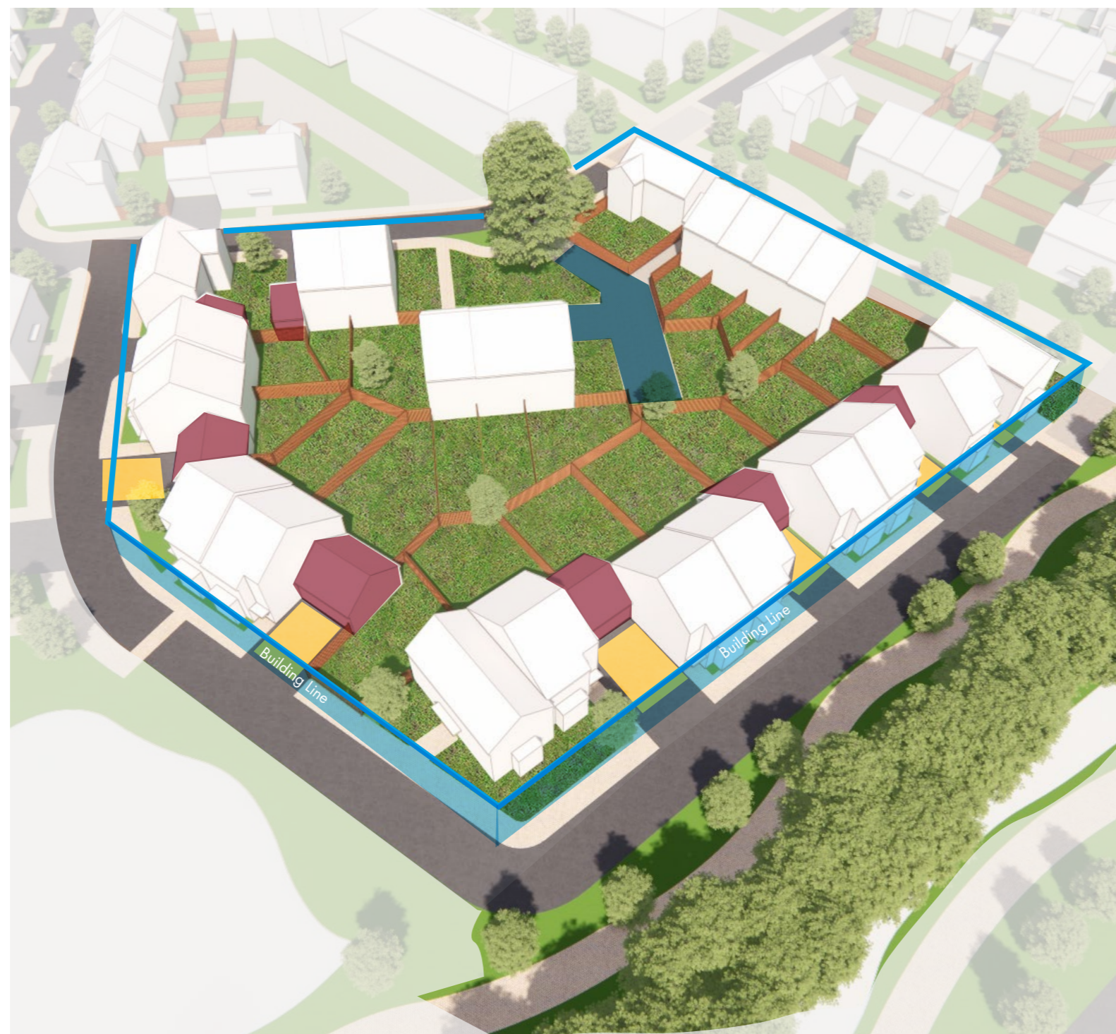
Typical Perimeter Block & Parking Arrangement
